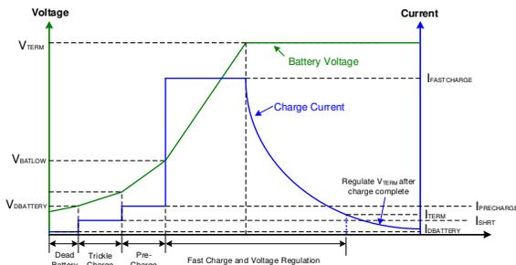
**Figure 10: Battery Charging Profile**
