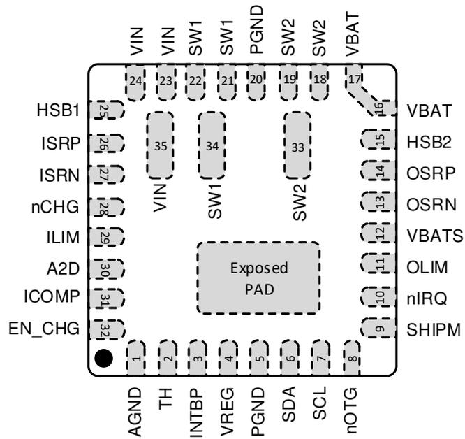
Figure 1: Pin Configuration – Top View – QFN4x4-32
