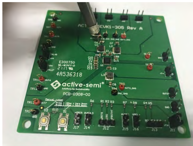
Figure 4—Measuring output voltage ripple
