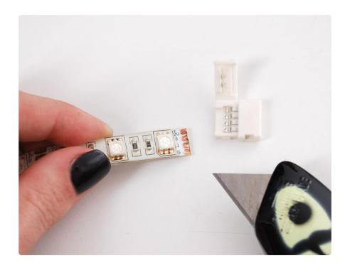
Use a utility knife or other sharp blade to carefully remove the plastic coating on the end of your RGB LED strip. You will need to make one cut perpendicular to the strip (like slicing a loaf of bread), being careful to only cut through the clear rubbery plastic and not the actual circuit, and then another cut along the surface of the circuit, with the blade oriented as shown above. This will expose the copper pads and make a skinny tab we can slide inside the solderless clip.
