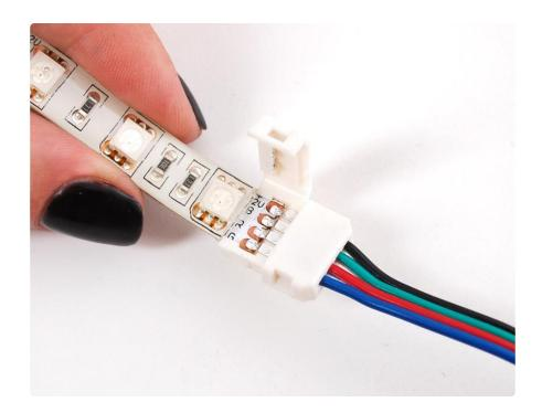
Open the plastic cover on the clip and slide the freshly sliced end of RGB LED strip under the metal tabs inside the connector.
