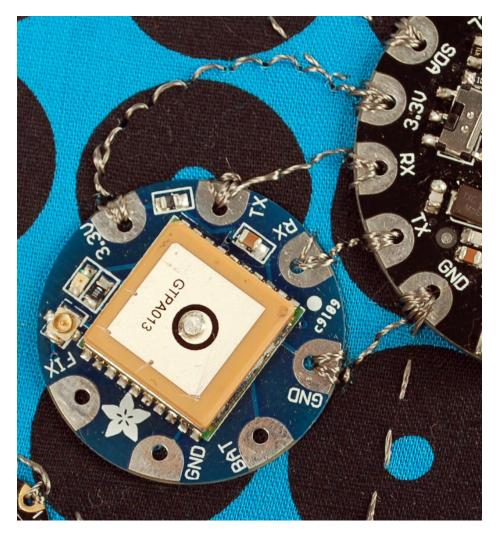
The four connectors are all in a row just to the left of Flora's JST battery connector for easy sewing. But test your project with alligator clips before sewing it in!
