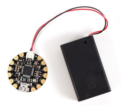
After loading your program onto the FLORA, you'll want to unplug the USB cable and go portable with battery power! USB will always power the board, but battery power (through the JST connector) can be turned on and off with Flora's onboard switch (near the "ON" text on the board). We recommend our <u>3xAAA holder</u> (http://adafru.it/ 727) for beginners, which conveniently plugs into FLORAs JST port.
