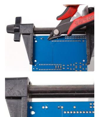
Once the soldering is complete, we can clean up by clipping the leads of the resistor. This keeps them from shorting to something else. Use diagonal or flush cutters to clip the wires right above where the solder joint ends.
