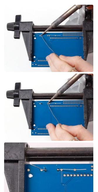
Bend the 'legs' of the resistor out so it sits flat against the PCB and flip it over.
