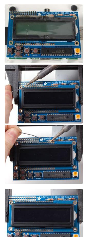
Slide the LCD over the header so that it is perfectly centered over the four holes and the silkscreen.
