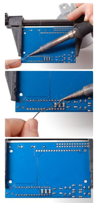
Flip over the PCB and solder in the 28 pins of the port expander.
