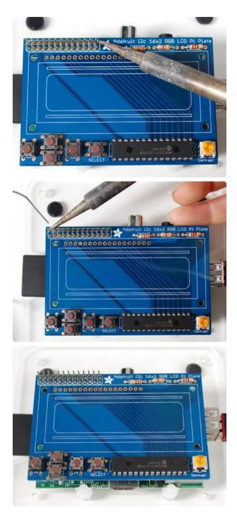
Now we will solder all 26 pins for the plate - this will send power and data between the two boards and also provide a mechanical stability. You may need to hold the plate down with tape to get it sitting flat against the Pi.
