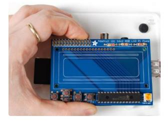
Place the 2x13 header onto your Pi, and slide the plate on top, it should fit perfectly.
