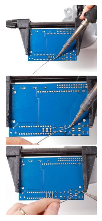
Flip over the PCB and check that all the legs for the buttons are sticking out.
