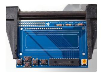
We're nearly done! Now we will place the I2C port expander chip. Double check that it has the MCP23017-E/SP marking on it. This is a 16-pin expander chip, that uses the i2c bus. That means you can send it commands using the i2c pins on an Pi and control 16 more digital pins! 5 of those pins go to the buttons, 6 go to the LCD control and 3 are used for the backlight (the remaining 2 are unused).
