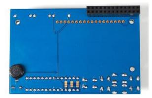
Flip over the assembly, carefully. Then solder in the 16 or 18 pins of header
