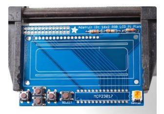
Next, place the 10K potentiometer (the orange-faced thing with three legs) into the spot above the RESET button. It will only fit one way. This is the contrast potentiometer which will adjust how dark the characters appear. All displays are slightly different so you'll adjust this once the display is soldered in.
