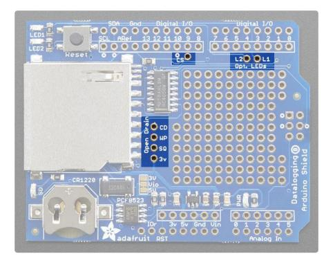
We also have some extra breakouts shown above, around the breakout board area.
