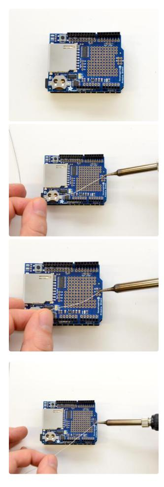
Place the board on the Metro and solder the 2x3 header
