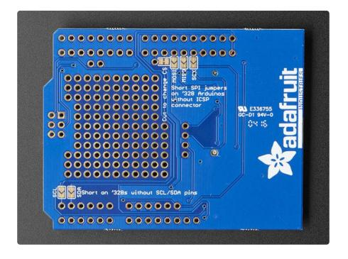
If you are using the shield with a 3.3V logic Arduino, you may want to change the Vio jumper. This is what the 10K pullups for I2C are pulled up to. Honestly, the pullups are very weak so if you forget, it's not a big deal. But if you can, cut the small trace between the center pad and 5V and solder the other side so that Vio is connected to 3V
