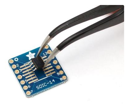
Nothing is as fast and fun as prototyping on a breadboard, but at some point you will find that the chips you want to work with are only available in non-breadboard-friendly SMT/SMD (Surface Mount Technology/Surface Mount Device). Unlike most DIP chips and resistors, SMT parts do not have the leads going through holes in the PCB. Instead, they 'float' on top, with often-rectangular solder pads.
