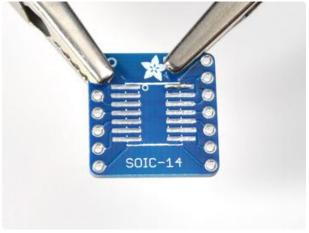
Next you need to place the part onto the pads, and you'll want to get the orientation right. You can look for a dot (indicating pin #1). In some cases, look for a flattened corner (on the left side here) which indicates which side is on the left
