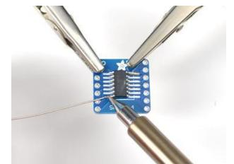
Now you can 'fix' the chip in place by soldering in the opposite corner. The one pin you soldered will keep the chip in place mostly, so you just have to solder the other pin a little to make the setup secure
