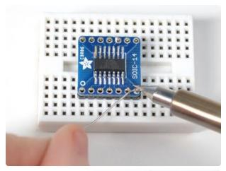
Almost done, now all you have to do is solder each header pin into the corresponding hole to make a secure connection
