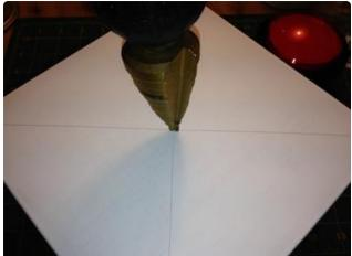
The massive arcade button needs a 1" circular hole cut. Measure to find the center line of your box. Using a step drill bit, drill down until you reach 1".
