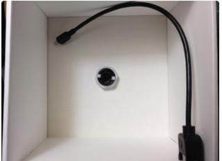
Next, install the massive arcade button on the top of the box. Remove the white plastic locking nut on the bottom of the button. Place the button through the hole and tighten the locking nut from below.
