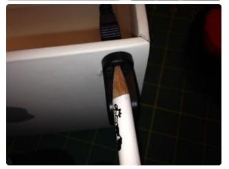
Now drill the hole for the USB port, locating it on the back, lower right of the box using a 1/2" circular hole. Next, drill the two holes for the mounting ears that hold the USB port in place. The mounting ear holes are ~28.5mm apart.
