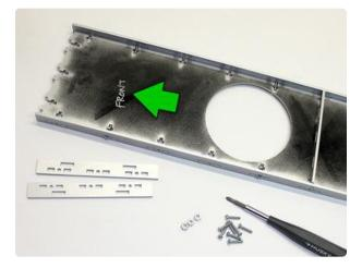
The spine, middle separator and the frame sides are joined using 1/2" #4-40 screws and nuts (20 total). About \$3. The top and bottom edges will be added shortly.
