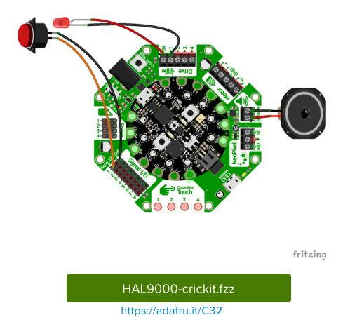
Attach the alligator clips to the button terminals as shown.
