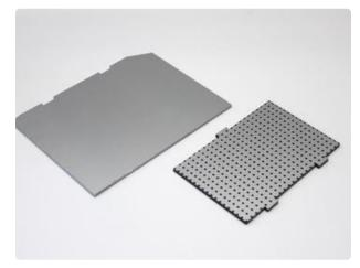
The speaker grille required its own set of hoops to jump through: all those tiny holes would be time-consuming and error prone (laser-cut holes tend to stick in place). Instead, a scrap of black acrylic was painted before cutting, then the laser was used to etch the surface and reveal the black plastic underneath those spots before the final perimeter cut.
