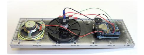
The Wave Shield includes solder holes adjacent to each Arduino header pin, allowing wires to be added. Remove the shield from the Arduino, insert wires from above and solder on the underside. The following connections are made:
