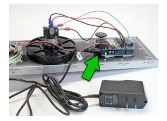
The 9V power source (whether battery or AC adapter) connects to the DC jack on the Arduino board.
