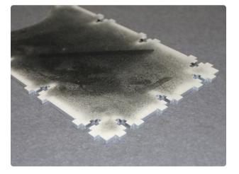
Here are the frame pieces after painting. The ruler is there as a point of reference: notice how "wavy" these pieces are; narrow pieces laser-cut from black acrylic seem particularly susceptible to this. The plethora of screw holes help hold everything flat once assembled.
