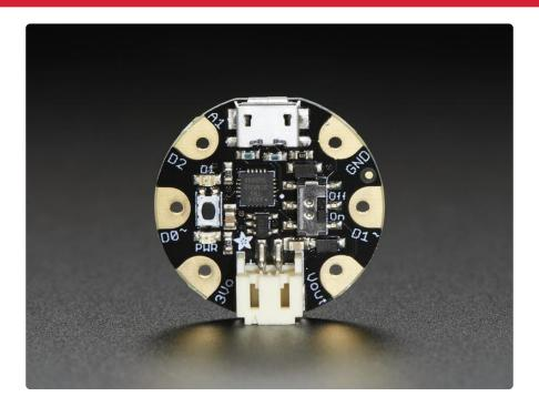
Don't forget to plug in the Gemma via a known-good USB cable to start the process. You should see the green power LED lit and the red bootloading LED pulse indicating that the Gemma is ready to start programming. If you've programmed the Gemma since getting it, you can always get it back to the bootloader state by pressing the small onboard reset button.
