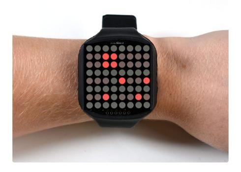
64 LEDs light up to tell you the time in a variety of ways. Built into the kit are 3 different watch 'faces' - a scrolling marquee with time and date, a binary watch display (for geeks, robots and binary fans), and a moon phase display (for beach-combers,
