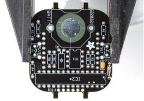
Ceramic capacitors, like resistors, are not directional. So put it in any way it fits, next to the R10 resistor, so its surrounded by the C1 outline
