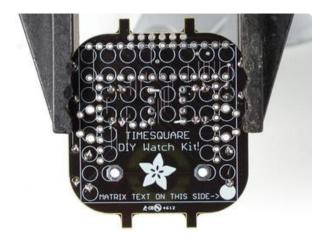
Next up we will put in the first chip. This chip has 8 legs and has the label DS1337 on top. Make sure you've got the right label on the chip.
