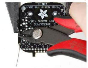
Next we'll solder in the yellow blobby 0.1uF capacitor. This capacitor is part of the reset circuitry as well, and is used to help reset the chip when we want to reprogram it.
