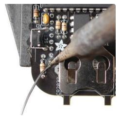
Now solder in all the pins of the matrix, you may have to angle the iron tip a bit to avoid burning other parts
