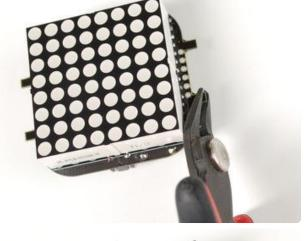
After you've assembled your watch there are a few ways to change the fit of the band around the PCB. First is trimming down the nubs on the PCB. These are there to help keep the board inside the rubber band. However, they may be long depending on your wrist size, and band (all the bands are slightly different)
