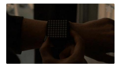
This is a DIY kit, and requires some basic soldering/assembly to put together. It is a beginner kit, so this is a fine project to use in learning how to solder. Tools are not included, you'll need a soldering iron, solder and diagonal cutters as a minimum. Che ck the tutorial page for details on what tools and steps are required to assemble. (htt ps://adafru.it/aTa) Take about 1-2 hours to put together. Build it in the afternoon and you'll be done in time to hit the clubs in the evening.
