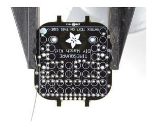
Bend the wire leads out so the resistor sits flat against the PCB. Then you can flip it over and it wont fall out!
