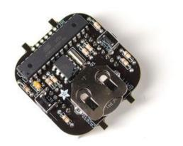
Insert a 20mm (CR2032) coin cell battery so that the flat + side is facing up and the bumpy side is facing down into the PCB
