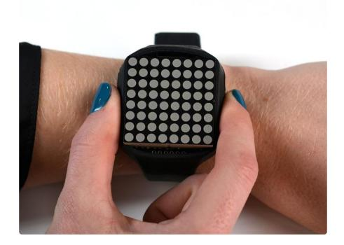
First wake the watch by tapping either side button. With the time display active, you can enter time-setting mode by holding down both side buttons for about two seconds. If using the watch for the first time, or after swapping batteries, it may wake in time-setting mode automatically.
