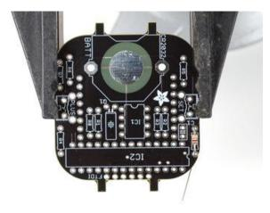
Start by placing the PCB in a vise to keep it steady. We'll be soldering parts on TOP, where the silkscreen shows the component placing. The first part we'll place is the 10K resistor. This resistor is marked brown black orange gold. (It's also the only single resistor of that color)
