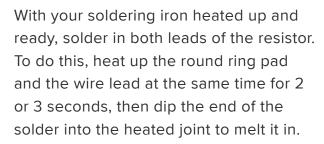
Then remove the solder and the soldering iron.
