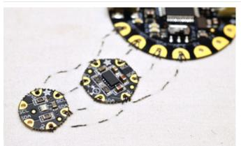
Stitching the sensor into a project is easy-- just line up the sensor so its adjacent to the SDA/SCL pins on Flora or another I2C sensor, and stitch the four connections with conductive thread. This is covered in more detail in the Flora Accelerometer (https://adafru.it/aYS) guide and our Conductive Thread (https://adafru.it/aVx) guide.
