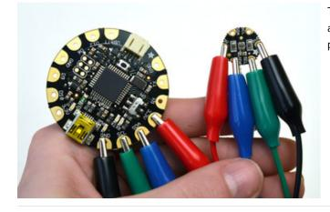
To test the sensor before sewing it into a project, use alligator clips to hook up the 3.3v, SDA, SCL, and GND pins.
