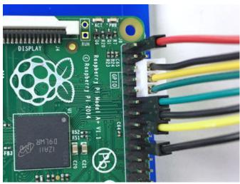
For the 2017-and-later kit, plug in the connections as shown here.
