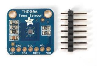
Unlike most temperature sensors, the TMP006 does not require contact with the object it is measuring. It uses a very sensitive thermopile to measure the infrared energy being emitted from the surface of the object.
