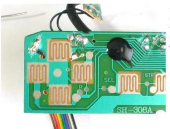
OK lets solder to the first button. The key is to remember to NOT solder to the same common pad but to the *opposite* pad! Solder the white wire to the 'up' button. There's almost always a hole you can feed the wire through!
