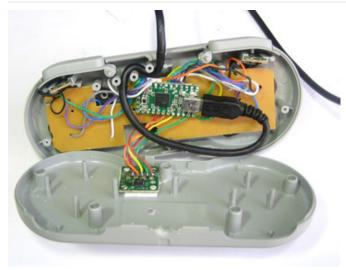
Finally, twist the USB cable so that it goes through the strain relief posts. If this makes it really tough to close you can probably skip it and just be careful not to yank!
