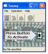
Press the tiny button to start the bootloader, so that it looks like this:
