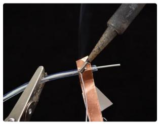
Heat up your soldering iron to 650 degrees F and make sure its hot by melting solder onto the tip, it should melt easily. Now press the tip of the iron to the two wires and copper tape and quickly dab some solder in. Then remove the iron. This should not take more than a second or two or the EL wire casing will melt.
