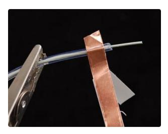
Unwrap a few mm of tape from the backing and stick it right next to the edge of the stripped EL wire. Fold the two thin wires on top.
