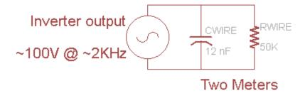
The capacitance and resistance per meter depends on the 'thickness' of the EL wire, the brand and make, the voltage and frequency applied
