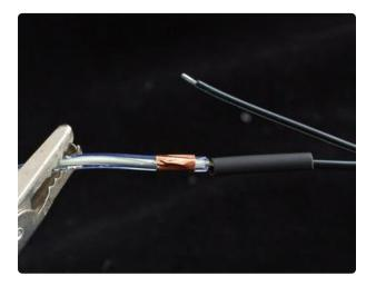
After 15 seconds check that the solder connection has cooled, then slide the 1/8" shrink over the middle joint.
