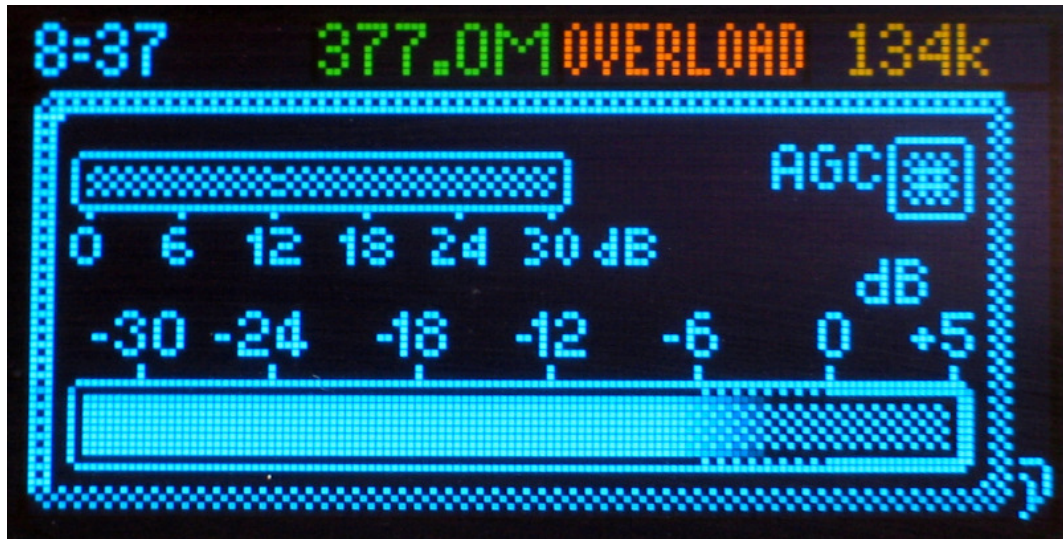
Figure 3: Real record display with monochrome VU meter.
