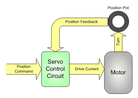
The problem with controlling a standard RC servo motor from a microcontroller is that it is 'closed loop' inside the servo motor case, but 'open loop' with respect to your microcontroller. You can tell the servo control circuit how you want the shaft positioned, but you have no way to confirm if or when this actually happens.
