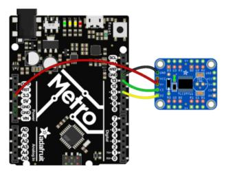
Connect VCC and V+ together to 3.3V (if a 4V+ power source is not available)
