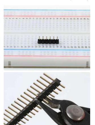
Position the header Cut to size first if necessary
