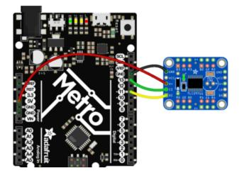
Keep VCC disconnected, and connect V+ to 4-17V
