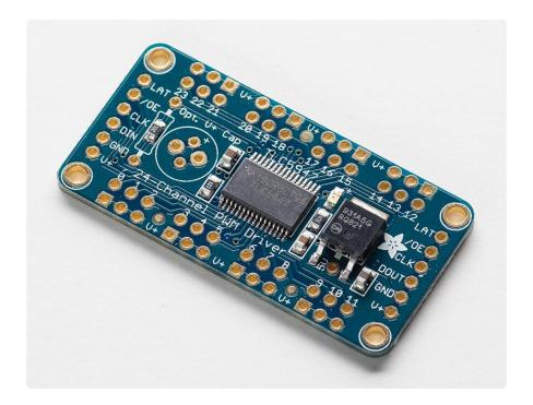
Both boards have a 2 or 3-pin SPI interface. Our library lets you use any two (TLC59711) or three (TLC5947) free pins to drive them. Best of all, you can chain multiple boards together to control hundreds or thousands of LEDs!
