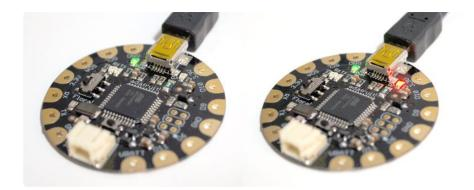
That's it! The on board LED marked "D7" should blink on and off repeatedly, and you've successfully programmed your FLORA!
