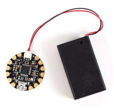
After loading your program onto the FLORA, you'll want to unplug the USB cable and go portable with battery power! USB will always power the board, but battery power (through the JST connector) can be turned on and off with Flora's onboard switch (near the "ON" text on the board). We recommend our <a href="mailto:3xAAA holder">3xAAA holder</a> (http://adafru.it/727) for beginners, which conveniently plugs into FLORAs JST port.
