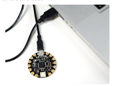
Next it's time to load up a program on your FLORA. There is an LED on board, so let's blink it! Plug in the USB cable and paste the following code into the Adafruit Flora IDE:
