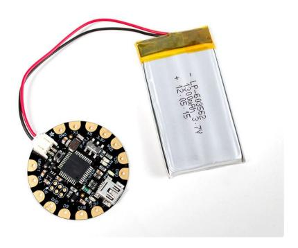
More advanced users may wish to use a rechargeable <u>lithium polymer battery</u> (http://adafru.it/258) for their smaller size and longer duration. These batteries pose added risk if abused, shorted, bent, crushed, or punctured. FLORA does not have onboard charging, so you would also need a separate <u>LiPoly charger</u> (http://adafru.it/259).
