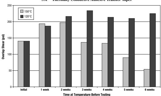
3M<sup>TM</sup> Thermally Conductive Adhesive Transfer Tapes
