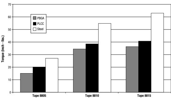
3M<sup>TM</sup> Thermally Conductive Adhesive Transfer Tapes
