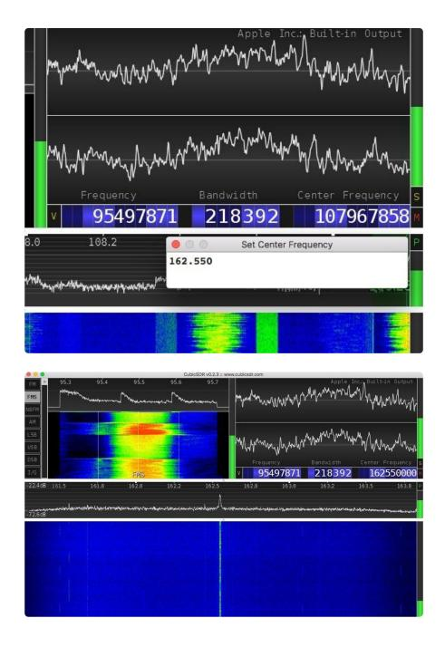
You can see a little peak, its much smaller signal than the FM radio stations. It's also much thinner which makes it a narrow-band FM rather than wideband. Since it's voice, not stereo music, they use less of the frequency band, so select NFM as the decoding type.
