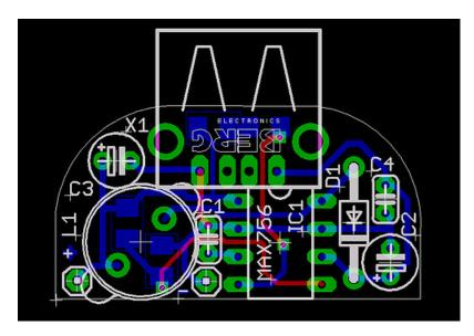
I actually do another etch test, to verify eveything one last time. Then I tile two boards together (cheaper) and generate gerbers.
