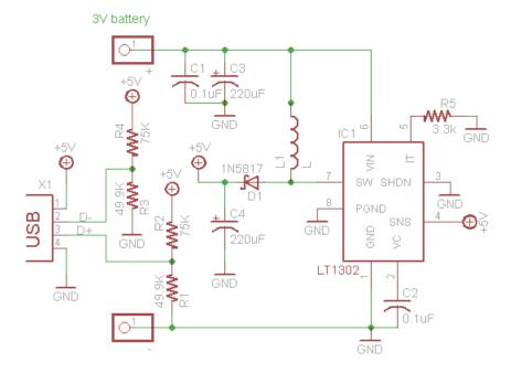
To improve compatibility with the latest smartphones and Apple devices, the charging protocol was reverse engineered so that the Mintyboost would be more universal. The pullup/down pins were also changed a full resistive divider which made it work with LiPoly batteries and Apple devices (https://adafru.it/c3k). Still uses a LT1302 chip.
