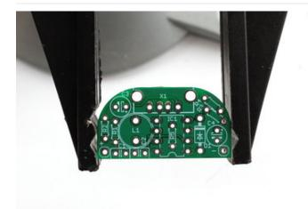
Place the PCB in a vise, and turn on the soldering iron.
