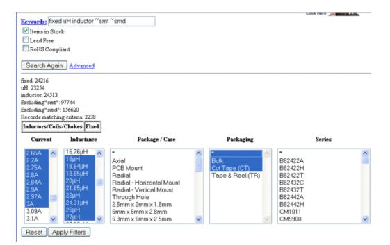
That filters it down to about a dozen choices. The SLF inductor is actually surface mount, and we're going to outright ignore the ones that cost more than \$2.50. Inductors for small electronics like this should cost around \$1-\$2, as a guideline. That leaves us with the DN7418-ND "INDUCTOR 27UH POWER AXIAL" and the 6000-220K-RC "INDUCTOR HI CURRENT RADIAL 22UH." Both of these look good, with about ~1.5A saturation current and 0.07 ohm DC resistance.
