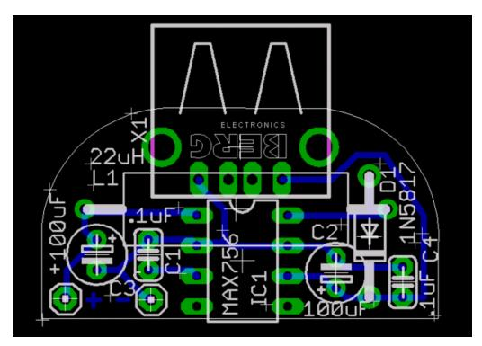
Since I am know this is just a prototype version, I make the PCB single sided -- for easy etching. I also make the traces really large.
