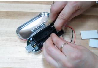
Try a test fit. Slide the board in first, then fit the battery pack in. Don't put the batteries in for this test! The circuit board could short against the tin and destroy the circuit!
