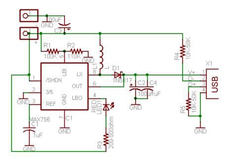
After a few months it became clear that some devices especially Apple music players, needed pullup/down resistors, so a new version that could fit 1 pullup and 1 pulldown was designed. This version still used the MAX756 (https://adafru.it/c3T).
