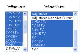
Looking over this list, it looks like I have a lot of options so I'm going to go back and select only the chips that can be preset to 5V (as opposed to adjustable ones that use 2 resistors to set the voltage). 5V is very common so every reasonable DC/DC chip will be available with such an option.
