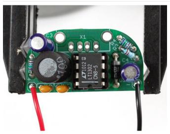
Finally, carefully insert the boost converter chip. Make sure the notch in the chip matches the notch in the socket. If the socket was inserted backwards, make sure the notch faces the flat edge of the PCB as shown. Make sure the chip is seated all the way in and that the pins aren't bent.
