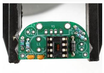
Next is the IC socket. This protects the chip and allows you to replace it if there are any problems. The socket goes *over* the 3.3K resistor but the resistor should not interfere as long as it was soldered in properly.
