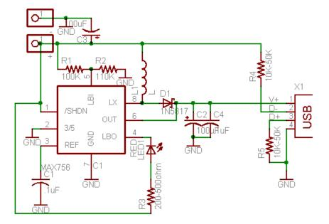
Note that because the mintyboost runs from 2 AA batteries, we can get 3V directly from the batteries so we connected the pullup right to the battery input.
