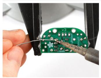
The socket has short legs so it can be annoying to keep in the right position. Hold it in place with one finger and 'tack solder' a corner.
