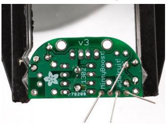
The next type of part we'll place is the ceramic capacitor. These are parts C1 and C2. Ceramic capacitors have a nice property that they are symmetric/non-polarized. That means they can go in 'either way'. Place the capacitor so that the 2 legs (leads) slide thru the two metal holes in the PCB (pads). The capacitor will sit flat against the PCB.
