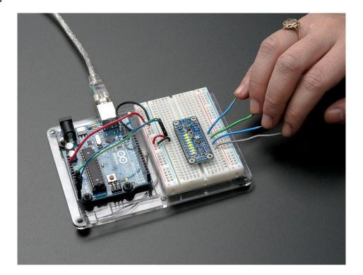
Add lots of touch sensors to your next microcontroller project with this easy-to-use 8-channel capacitive touch sensor breakout board, starring the CAP1188. This chip can handle up to 8 individual touch pads, and has a very nice feature that makes it stand out for us: it will light up the 8 onboard LEDs when the matching touch sensor fires to help you debug your sensor setup.
