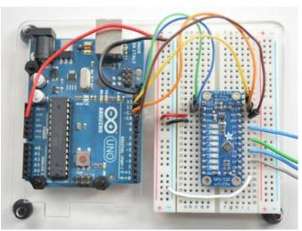
Connect **Vin** to 5V and **GND** to ground, then tie a wire from **AD** to ground as well. Now connect the **SCK**, **MISO**, **MOSI**, **CS** and **RST** pins to your microcontroller. If using an Arduino you can use either the hardware SPI pins which are fixed for each Arduino, or go with software SPI where you select any 5 digital I/O pins
