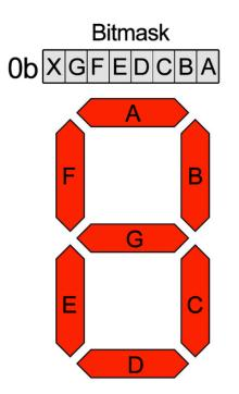
The bitmask is a single 8-bit number that can be passed in as a single Hexidecimal, Decimal, or binary number. This will use a couple different methods to display **8E8E**:
