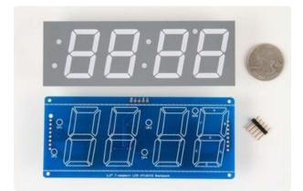
When you buy a pack from Adafruit, it comes with the fully tested and assembled backpack as well as a 7segment display in one of the colors we provide (say, red, yellow, blue or green). You'll need to solder the matrix onto the backpack but its an easy task.
