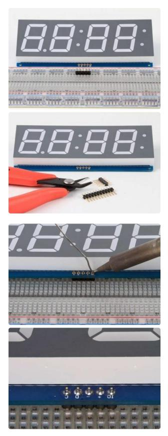
Cut the header strip to length if necessary and insert LONG pins down into the breadboard.
