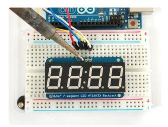
Place the soldered backpack on top of the header and Solder 'em!
