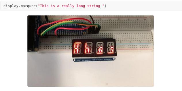
By default it is 0.25 seconds, but you can change this by providing a second parameter. You can optionally pass **False** for a third parameter if you would not like to have it loop. So if you wanted each character to display for half a second and didn't want it to loop, you would use the following:
