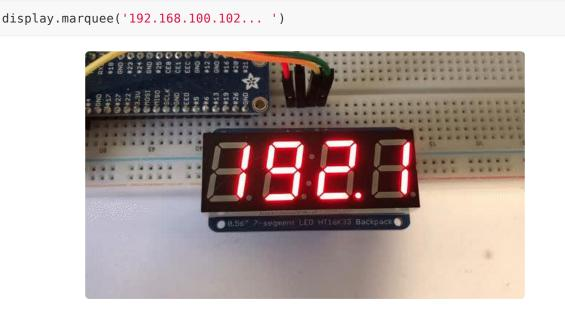
By default it is 0.25 seconds, but you can change this by providing a second parameter. You can optionally pass **False** for a third parameter if you would not like to have it loop. So if you wanted each character to display for half a second and didn't want it to loop, you would use the following:
