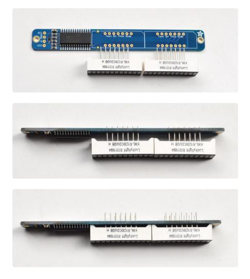
To keep the two bargraphs lined up nicely, you can use a little masking or scotch tape on the bargraph modules, tape them so they are in a straight line. There is a little play during soldering so if you don't do this the two modules may not be in a perfect line.
