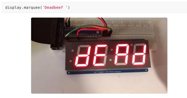
By default it is 0.25 seconds, but you can change this by providing a second parameter. You can optionally pass **False** for a third parameter if you would not like to have it loop. So if you wanted each character to display for half a second and didn't want it to loop, you would use the following:
