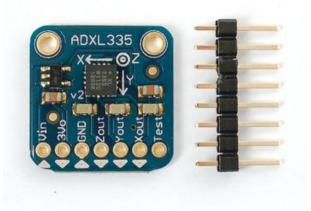
The ADXL335 can measure at least +/-3G in the X, Y and Z axis. It is perfect for high-resolution static acceleration measurements such as tilt-sensing, as well as for moderate dynamic accelerations from motion, shock or vibration.
