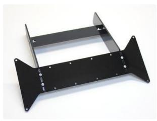
The "bow tie" now joins with the legs, using the same t-slot technique with four #4-40 1/2" screws and nuts.
