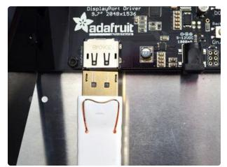
OK plug in your cable so that it snaps in nicely into the DP connector on the Qualia driver. It should snap in all the way
