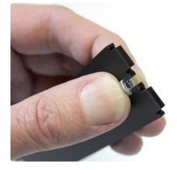
Slots in the leg pieces are "keyed" to fit into the tabs on the cross brace. Position a leg using these tabs and slots, then install a #4-40 1/2" screw through the middle, meeting up with the nut held in the cross brace.
