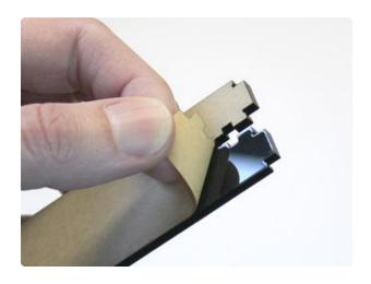
Start by peeling the backing paper off both sides of all the laser-cut parts. It's easiest to start at a corner, catching the edge of the paper with a fingernail.
