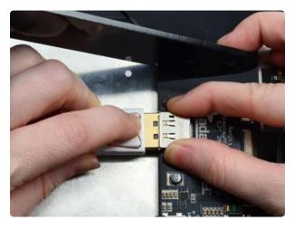
Removing a DisplayPort connector is a little more difficult because the connector is quite strong. You have to press down on the cable latch and wiggle-pull it out. Hold onto the connector with your other hand to make it easier!
