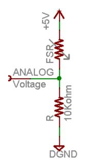
For this example I'm showing it with a 5V supply but note that you can use this with a 3.3v supply just as easily. In this configuration the analog voltage reading ranges from 0V (ground) to about 5V (or about the same as the power supply voltage).
