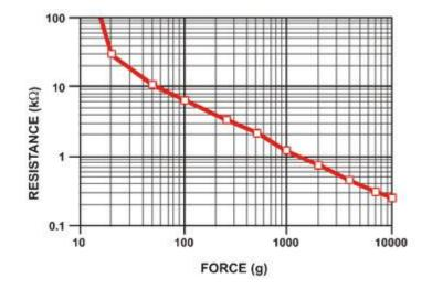
It is important to notice that the graph isn't really linear (its a log/log graph) and that at especially low force measurements it quickly goes from infinite to  $100 \text{K}\Omega$ .
