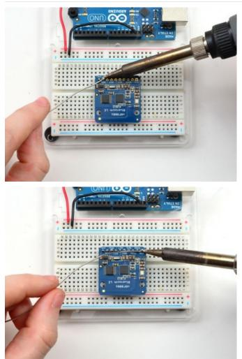
And Solder! Be sure to solder all 10 pins for reliable electrical contact.
