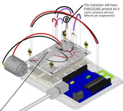
:NOTE: if your arduino is resetting you need to install the optional capacitor:.
