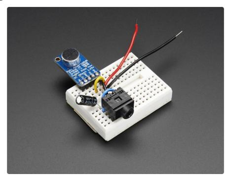
The microphone amp is thankfully quite simple to get started. No microcontroller or programming required. We suggest wiring it up directly with a battery pack and headphones to start while you get a hang of how the AGC acts and responds.
