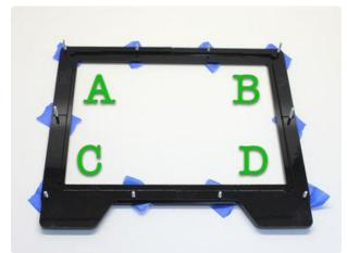
Slide each of the corner supports over the screws in the correct positions. The etched letter should be visible and in the correct orientation for reading. A at the top left, B at the top right, C at the bottom left, D at the bottom right.
