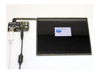
Optional: testing the LCD and driver board before assembly may avoid some troubleshooting later. Read ahead to the "How to Use" page for guidance.
