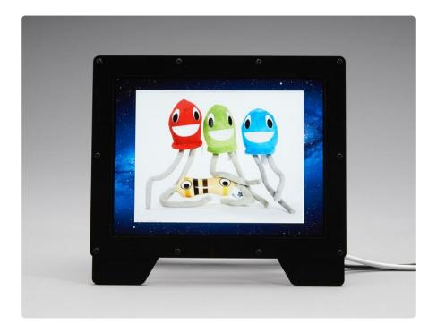
Using the Qualia display is super easy, similar to any other monitor you've used. You will need a 9 or 12V DC power supply that can provide at least 1000mA (1A) of current, a DisplayPort cable and a computer with a DisplayPort
