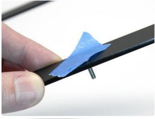
Insert a screw into each hole (1/2" or 5/8", as appropriate to the above diagram). The bezel will need to be flipped over later, so as you place each screw, secure it with a bit of tape, or you can use the nuts temporarily to keep the screws from sliding out (you'll need to remove these nuts later).
