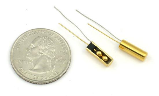
Tilt switches used to be made exclusively of mercury, but are rarer now since they are recognized as being extremely toxic. The benefits of mercury is that the blob is dense enough that it doesnt bounce and so the switch isnt susceptible to vibrations. On the other hand, ball-type sensors are easy to make, wont shatter, and pose no risk of pollution.
