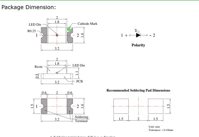
Soldering terminal may shift in x, y direction.
