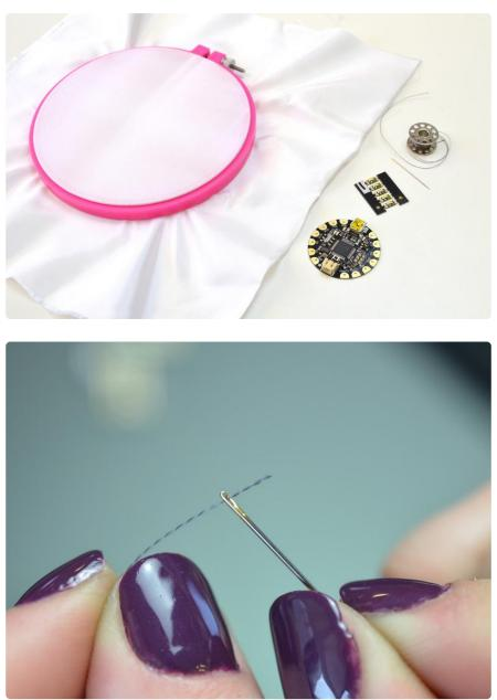
Grab a needle and test it's small enough to pass through the holes in the sequins. Thread up your needle with conductive thread, our 2-ply and 3-ply both are great for this purpose. <u>Check out our conductive thread guide</u> (https://adafru.it/aVx) to learn more about this stainless steel fiber.
