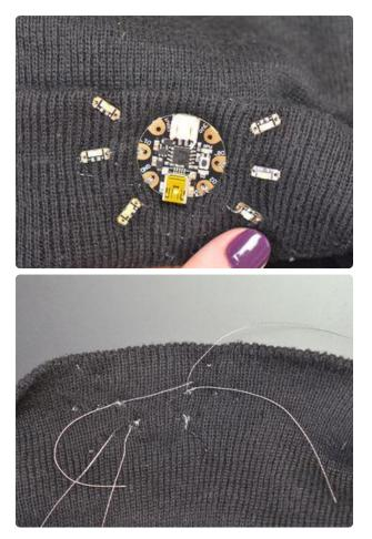
Next hook up the + connections from each of GEMMA's outputs to three pixels. We stitched from one sequin to the GEMMA, then over to another sequin and on to the third sequin before going back to the first, making a sort of square that results in the thread tails being in the same place.
