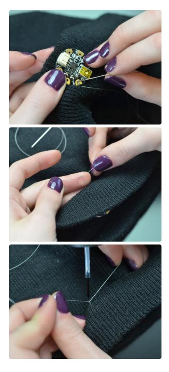
You can start with the pixel + or -. For this hat we chose to start with the shared ground line that hooks up all the sequins. Stitch around the GND pad on GEMMA at the edge of a knit cap and knot/seal at the back.
