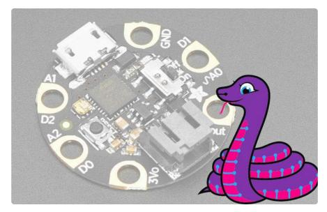
GEMMA M0 boards can run CircuitPython — a different approach to programming compared to Arduino sketches. In fact, CircuitPython comes factory pre-loaded on GEMMA M0. If you've overwritten it with an Arduino sketch, or just want to learn the basics of setting up and using CircuitPython, this is explained in the Adafruit GEMMA M0 guide (https://adafru.it/z1B).
