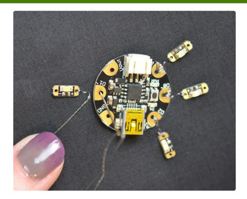
Avoid using pin D1 when using the Gemma M0. Instead use three LEDs in parallel on using pins D0 and D2.
