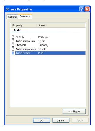
This file is 16KHz, 16-bit, mono PCM. Since thats below the maximum (22KHz, 16-bit, mono PCM) you are good to go. No need to convert the file.
