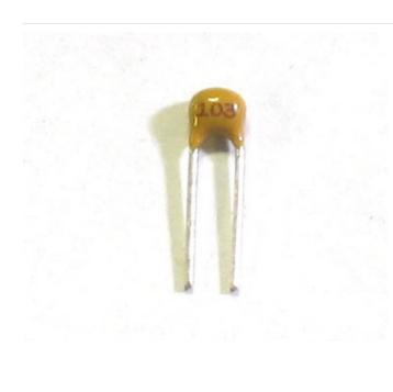
Next is the 0.01uF ceramic capacitor **C8**. The tricky part here is that in older kits there are many 0.1uF ceramic capacitors in the kit that look identical to the 0.01uF!
