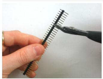
Next, break the 36-pin header strip into smaller sections so that the shield can be placed on the Arduino. You can use pliers or diagonal cutters. Clip off 2-6pin and 2-8pin pieces.
