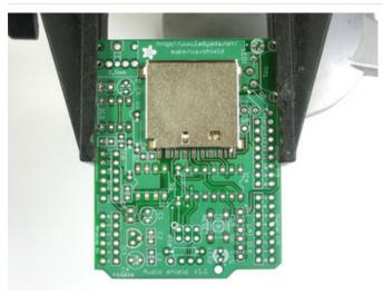
We're going to the SD card first. While surface mount parts are a little tougher than thru-hole, this piece has pin spacing of 0.1" so it is quite easy. Doing it first also gives us lots of working room.
