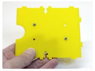
Locate the acrylic bottom piece and insert two #4-40 1/2" screws in the positions shown.
