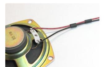
Solder one end of these wires to the connection points on the speaker.
