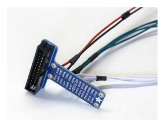
Add plain wires to the +5V and GND pins on the Cobbler (color-coded if you have them...if not, label these wires to avoid trouble).
