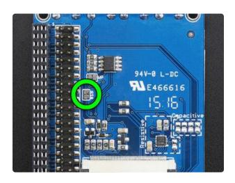
On the back of the PiTFT, near the GPIO pins, are two pads labeled "#18" with a narrow PCB trace between them.
