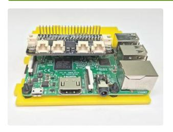
Install the Arcade Bonnet atop the Pi GPIO header as you did during the dry run.
