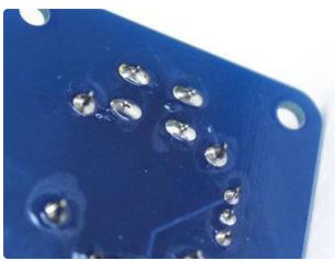
Make sure all your solder connections are smooth and clean, like tiny Hershey's Kisses®. There should be no solder balls or bridges, no gaps between pins and their corresponding pads.
