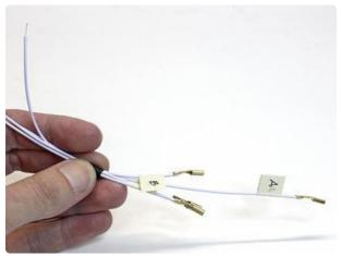
Now slide just <u>one wire</u> part way out, so we can tell it apart from the others at the bare end. Here we pulled the A wire and can identify its tail from the others.
