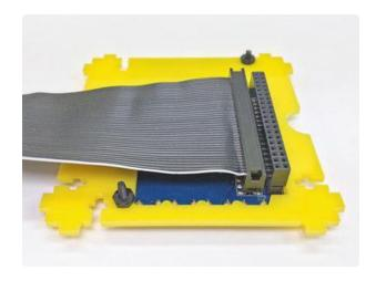
Plug one end of the 40-pin ribbon cable into the pin header on the back of the PiTFT.
