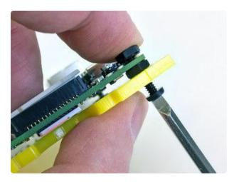
Instead, set a nut on the tip of one screw, and observe how it bumps up against nearby parts (such as the end of the GPIO header). You'll always find some orientation of the nut where it clears all the parts. Hold it in this orientation, then tighten the screw up from the bottom. The board will then be neatly sandwiched between the two nuts!
