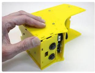
Stuff the credit/start button wires inside, then slot this piece into the holes on the "table" side of the case. Pivot it upright... tabs on the base should fit into holes on the front...and finally pop the last two tabs into the "loose" side.
