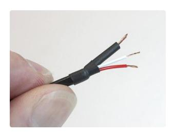
That bare copper wire on the audio cable is a problem...it connects to a ground point right next to a +5V line. We must insulate!
