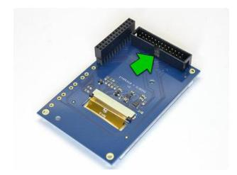
The tall female (socket) and shorter male (pin) headers will be installed in the positions shown. The female socket goes on the long edge of the PiTFT board, male on the short edge (labeled "Connector on reverse!" on the silkscreen side of the board).
