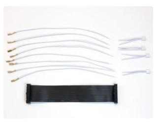
Clip the 2-pin plastic plugs off the button quick-connects. You should then have eight (8) wires with a metal spade on one end. Strip a little insulation from the other end.
