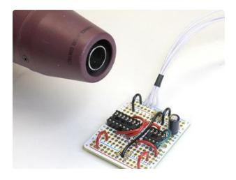
Now slide the heat-shrink back down the wires, about 3/4" from the board, and apply heat. Most people simply use a butane lighter for this, but if you have a heat gun that's even better.
