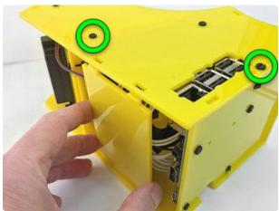
Get all the wires stuffed inside the case. Check the joystick jumper wires, which may have pulled free.
