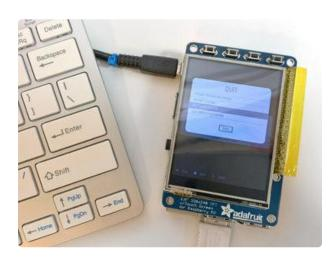
Install just the PiTFT display atop the Raspberry Pi, none of the other parts yet.
