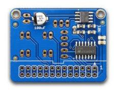
Generation 2 kits used the Cupcade Adapter Board with the 28-pin GPIO header as used on the Pi 1 Model B.
