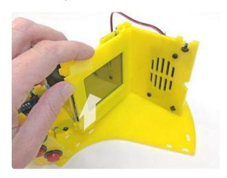
Pivot the screen support piece up slightly, fit the screen bezel into the slots on the speaker grille, and lower it all back into place.
