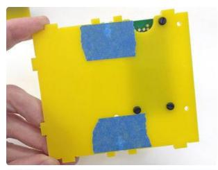
If using a Pi Zero, the sequence is a little different. Apply the tape first to the bottom face of the base piece, covering the two T-slots. Then, from above, slide a nut into each of the two slots. Really press them in to make sure they're making good contact with the tape.
