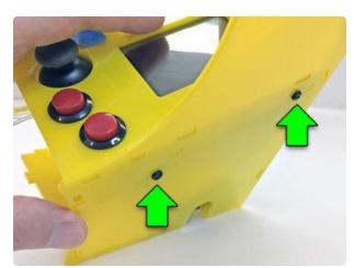
Fit the joystick and button supports into their own slots as you're working on this section. Use masking tape to hold these four pieces in alignment.
