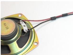
Solder two plain wires to the connection points on the speaker.
