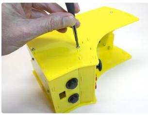
Loosen a side screw at the top. Same routine: screw tip flush with nut face, so you can flex this side up just a little bit.
