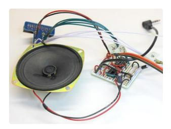
Solder the opposite end of the wires to the corresponding points on the amplifier circuit, then shrink the tubing near each end.
