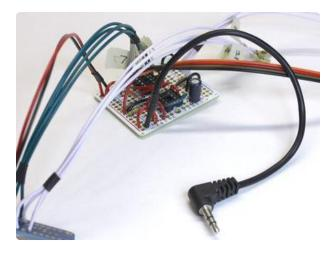
Solder the three wires to the proscribed locations on the Perma-Proto circuit.
