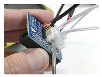
A small screwdriver is sometimes helpful when unplugging the buttons from the JST sockets. A little twist is usually sufficient...use common sense and be gentle.
