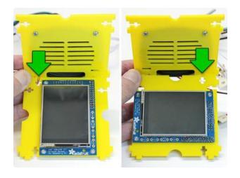
The screen fits into two slots at the bottom of the speaker grille.
