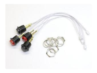
Remove all of the nuts and washers from the four buttons. You can leave the quickconnect wires attached.
