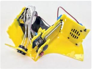
Take the jumble of parts and try to (roughly) align the tabs on the speaker grille, screen and joystick supports with the corresponding holes in the side piece. They probably won't stay in those holes for very long, but at least you'll know where they belong.
