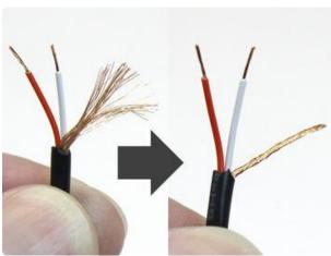
Strip 1/4" insulation from the two inner wires. Twist the stranded copper wire into a tidy bundle.
