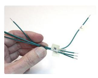
It's a very similar game with the U/D/L/R wires: squeeze them all through a piece of heat-shrink tube, then pull out one wire at a time, soldering the tail (unlabeled) end to the appropriate locations on the Cobbler...
