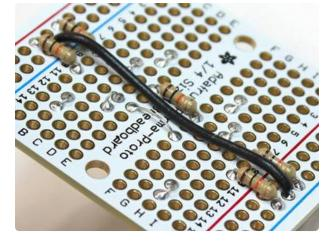
Eight short jumpers are now installed in the positions shown in pink. Most of these are very small, joining adjacent pads. We can use the un-insulated clippings from the prior step because no other conductive traces are crossed.
