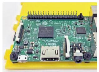
Here's how it looks when properly installed. Nuts are flush with both sides of the board, not pinching down on components. And the board is elevated at just the right height for the SD card slot and side cutouts to work.
