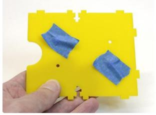
Add a piece of masking tape over each screw head to keep them from falling out.
