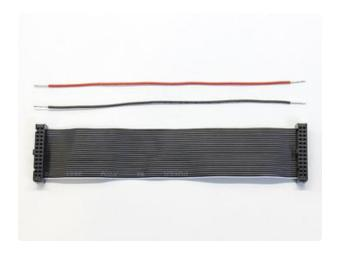
Cut two (2) wires about six inches long and strip about 1/4" of insulation from both ends.
