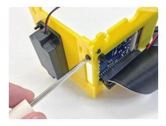
Bring the two pieces together and add a screw. This will pass through the plastic grille piece and into the nut.
