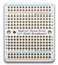
Generation 1 kits had you solder up several components and wires on an Adafruit Perma Proto board.
