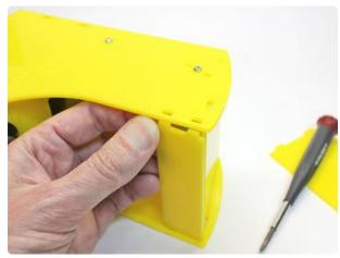
Slot the marquee into place, then retighten the top screw.
