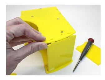
Insert the "roof" of the cabinet. The roof and back pieces are similar in size, but the tabs are spaced differently, so only the correct piece will fit.
