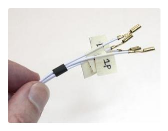
Now do a similar thing with the four labeled quick-connect wires. Slide a piece of heat-shrink as far along the wires as it will go.
