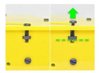
Idea is to loosen one or two of the screws nearest each piece as it's installed. Either right or left side of the case, doesn't matter. Sometimes both, if you need a little extra.
