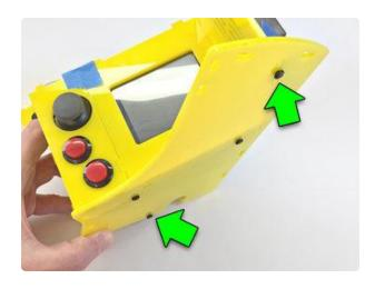
A third screw installs from the side at the top of the speaker grille piece.
