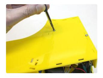
Work your way from bottom to top, aligning the tabs closest to each hole and then inserting a screw.
