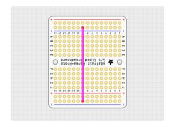
The Perma-Proto is turned around, with the labels upside-down. It's fine, this orientation just makes our circuit easier to lay out.
