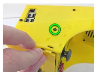
Loosen a screw and lift up the case side to install this front piece just below the joystick and buttons. There should be just enough clearance and flex for this to happen. Bend too far and you'll crack plastic or pop the head off a screw.
