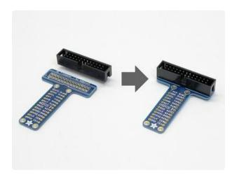
Install the male (pin) header on the Pi T-Cobbler.
