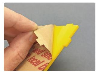
Peel the backing paper off both sides of all the laser-cut parts. It's easiest to start at a corner, catching the edge of the paper with a fingernail.
