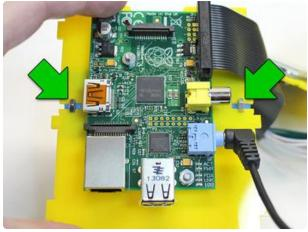
Then, from the top side, press a nut into the cross part of each "T." Give it a pinch from both sides, so the tape gets a good hold on the nut.
