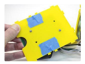
Put a piece of masking tape over each of the two T-slots on the underside of the base piece (where the Raspberry Pi is installed).
