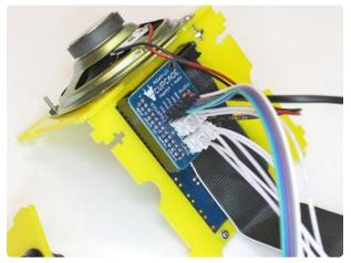
The Cupcade board plugs into the back of the PiTFT as it was during our dry run.
