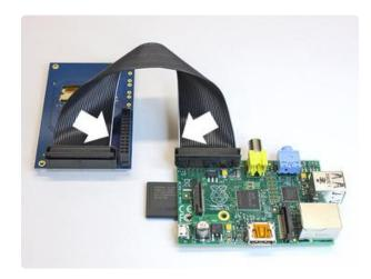
The header on the PiTFT is "keyed" so that pin 1 (the white wire) is always on the correct side. However, there's two ends to the cable. Plug in the end that places the cable running behind the PiTFT board, not out in the open.
