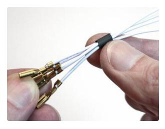
Slide the heat-shrink all the way down, near the metal spades, but don't shrink it yet!
