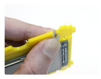
Bring the two pieces together and add a #4-40 1/2" screw. This will pass through the speaker frame, the plastic grille piece and into the nut.
