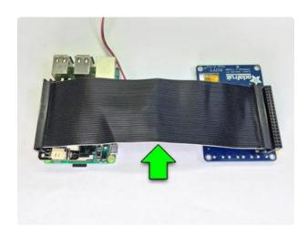
Disconnect the PiTFT from the Raspberry Pi, then plug the Arcade Bonnet in its place.
