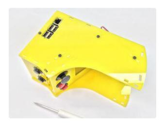
Work your way around the case, aligning the tabs closest to each hole and then inserting a screw, four in total.
