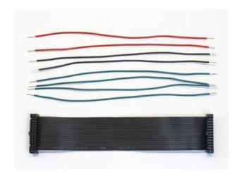
Cut eight (8) wires about six inches long and strip about 1/4" of insulation from both ends.
