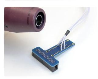
Slide the heat-shrink tube down close to the Cobbler and apply heat.
