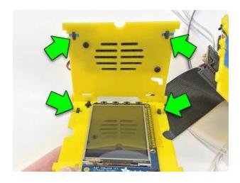
On the speaker/screen combo there's four T-slots total, two above the speaker, two above the screen.
