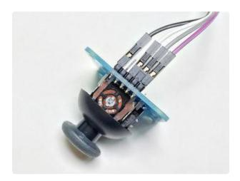
There are 5 pins on the joystick board, but only 4 jumper wires in the kit. Skip over the "Sel" pin...only the VCC, Xout, Yout and GND pins are used in Cupcade.
