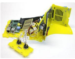
Take the jumble of parts and try to (roughly) align the tabs on the speaker grille, screen and joystick supports with the corresponding holes in the side piece. They probably won't stay in those holes for very long, but at least you'll know where they belong.
