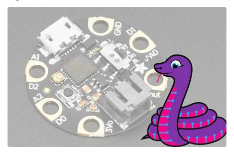
GEMMA M0 boards can run CircuitPython — a different approach to programming compared to Arduino sketches. In fact, CircuitPython comes factory pre-loaded on GEMMA M0. If you've overwritten it with an Arduino sketch, or just want to learn the basics of setting up and using CircuitPython, this is explained in the <a href="Adafruit">Adafruit</a> GEMMA M0 guide (https://adafru.it/z1B).
