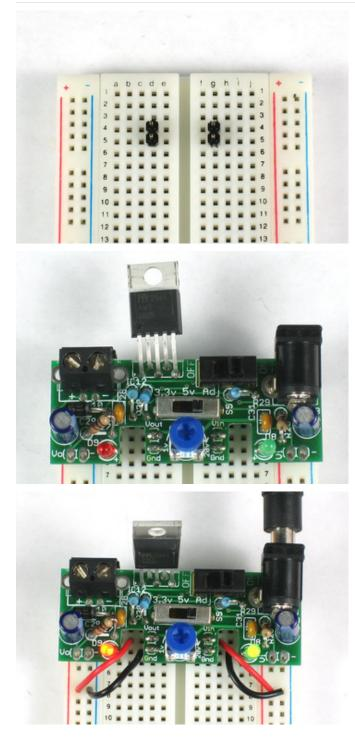
If your breadboard has nonstandard spacing, you can still plug it in using the header-breakouts in the middle.
