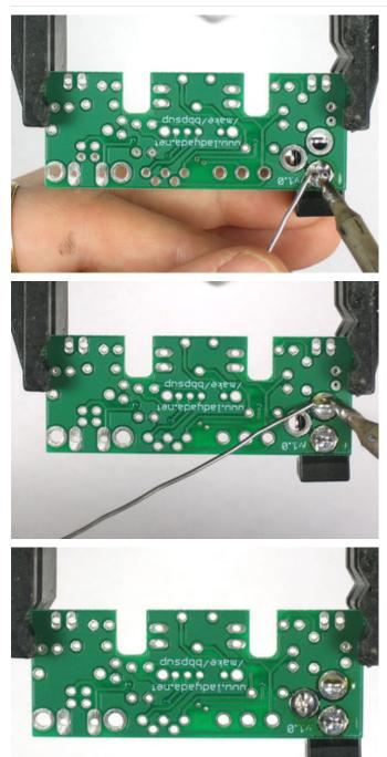
Flip over the PCB - you can either tape the DC jack down or use a finger to keep it place.
