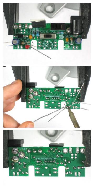
Finish off the 'low voltage' side by inserting the second 1.0K resistor **R2** and the second 0.1uF ceramic capacitor **C4**.
