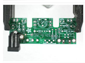
We'll start by placing the DC power jack. This is how we will attach outlet power supplies to the board. The jack is 2.1mm which is the most common size.
