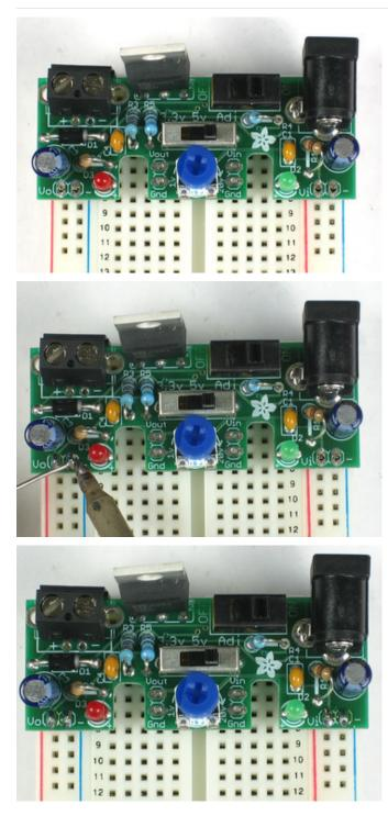
Now place the power supply on top. If it fits nicely, solder the four pins.
