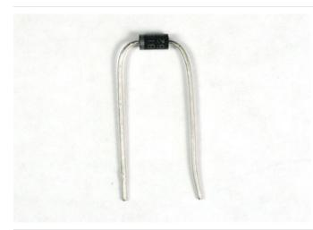
Next we will solder in the 1N5818 protection diode. Diodes only conduct electricity in one direction. This means we can use them to protect our circuitry from negative voltages - a top killer of electronics!
