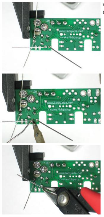
Bend the leads out so the parts sit flat against the PCB. Solder and clip the leads.
