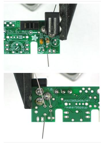
Place one of the 1.0K resistors (Brown Black Red Gold) into the slot marked R1. Then place right next to it one of the 0.1uF ceramic capacitors (they're small and yellow). The resistors and ceramic capacitors are non-polarized so they can go in 'either way'.
