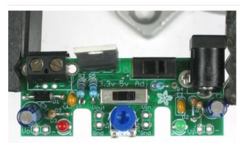
Next we will solder in the 2-pin terminal jack. This lets us connect up wires to power the board from a battery or similar.
