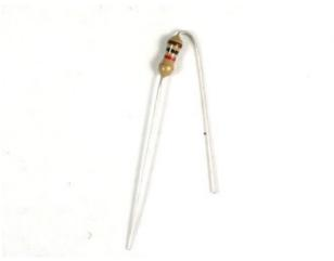
We're going to solder one of the 1.0K resistors in next. The resistors should be bent over 180 like shown. Note that resistors are 'non-polarized' so you can put them in 'either way' - they work the same forwards or backwards.
