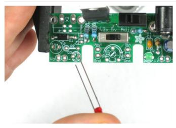
Now we will put in the capacitors and LEDs for the left hand "low voltage" side.
