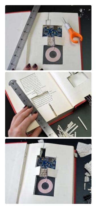
The coil should be as close to the cover as possible, but you might want to make the spot for the circuit a bit deeper so the USB connector is completely submerged in pages.
