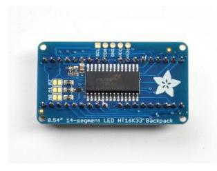
Check your work, making sure each pin is nicely soldered, and there's no cold solder joints or shorted pins
