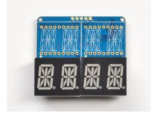
When you buy a pack from Adafruit, it comes with the fully tested and assembled backpack as well as two dual 14-segment display in one of the colors we provide (say, red, yellow, blue or green). You'll need to solder the matrix onto the backpack but it's an easy task.
