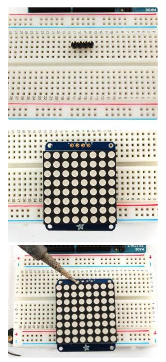
Now you're ready to wire it up to a microcontroller. We'll assume you want to use a 4pin header. You can also of course solder wires directly. Place a 4-pin piece of header with the LONG pins down into the breadboard.
