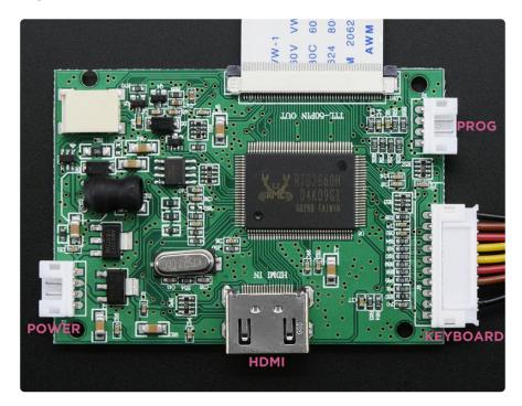
The PROG JST connect is generally for factory use only. It's the port we use to program the board before sending it to you
