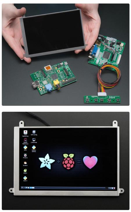
This is our smallest high-res display, with 1280x800 resolution. It's not IPS, however! We also have a version with HDMI audio support (PID #1695)
