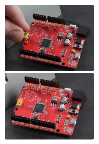
Install the 6-pin ICSP header from the Seeeduino kit from the top side and solder in place.
