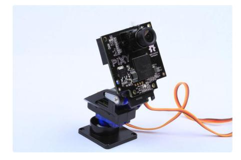
The Pixy Camera itself is fully assembled. We just need to attach it to the pan/tilt base and connect the servos.
