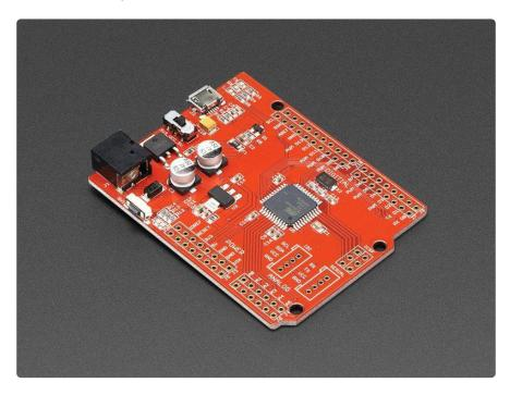
There is one little problem though. The Zumo chassis has a couple of unfortunately placed capacitors that interfere with the DC jack and capacitors on the Seeeduino. The good news is that the Seeeduino ships without headers installed. So all you need to do is replace them with slightly longer headers. The <u>Arduino R3 Stacking</u> Headers (http://adafru.it/85) are just the thing we need.
