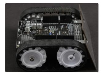
Plug the headers upside-down into the Zumo Chassis as shown.
