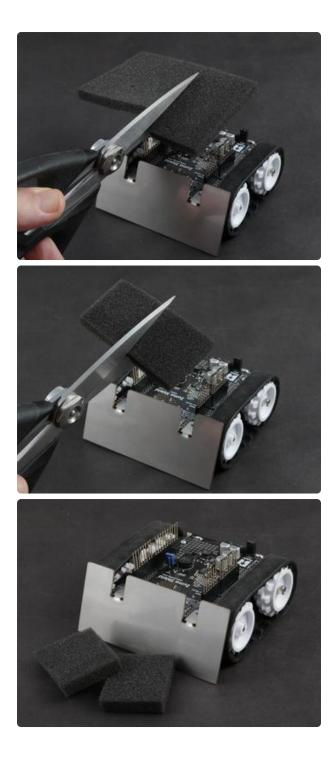
Using a piece of the packing foam from the Seeeduino kit, cut two small squares roughly 1.5"x1.5" (3.5cm x 3.5cm) - These dimensions are not super critical!
