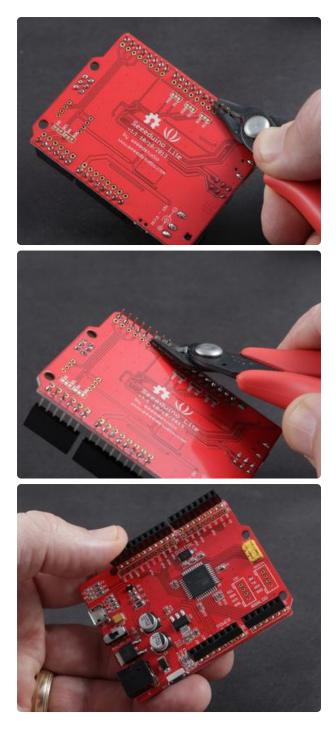
Trim the pins on the back and you are ready for the final assembly of your Pixy Pet!
