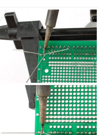
Solder both LEDs in place.
