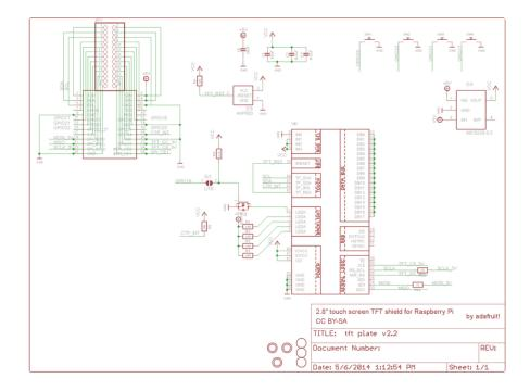
Schematic for PiTFT Plus (B+/Pi 2 shape)
