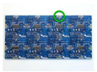
On the HELLA UNTZtrument — a 4x2 assembly of Trellises — connect the wires to the third header along the top edge, not the rightmost fourth header.
