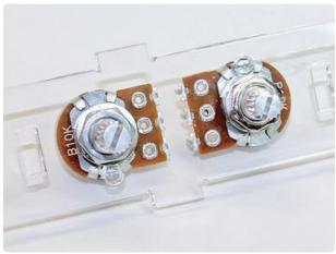
Potentiometers don't care which outer leg is ground or +V, but the choice does affect which direction has increasing output.
