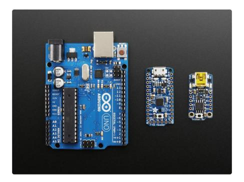
The Pro Trinket 5V uses the Atmega328P chip, which is the same core chip in the Arduino UNO/Duemilanove/Mini/etc. at the same speed and voltage. So you'll be happy to hear that not only is Pro Trinket programmable using the Arduino IDE as you already set up, but 99% of Arduino projects will work out of the box!
