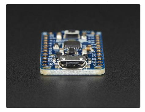
The Pro Trinket uses the Atmega328P chip, which is the same core chip in the Arduino UNO/Duemilanove/Mini/etc. It's the 'classic' Arduino chip! So you'll be happy to hear that not only is Pro Trinket programmable using the Arduino IDE as you already set up, but 99% of Arduino projects will work out of the box!
