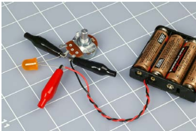
Figure P-1. Learning by discovery allows you to start building simple circuits right away, using a handful of cheap components, a few batteries, and some alligator clips.
